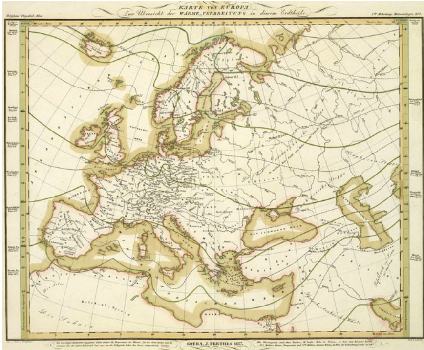
Fig. 3.7 Choropleths and isolines combined in a complex thematic map in Berghaus' atlas (1840)
