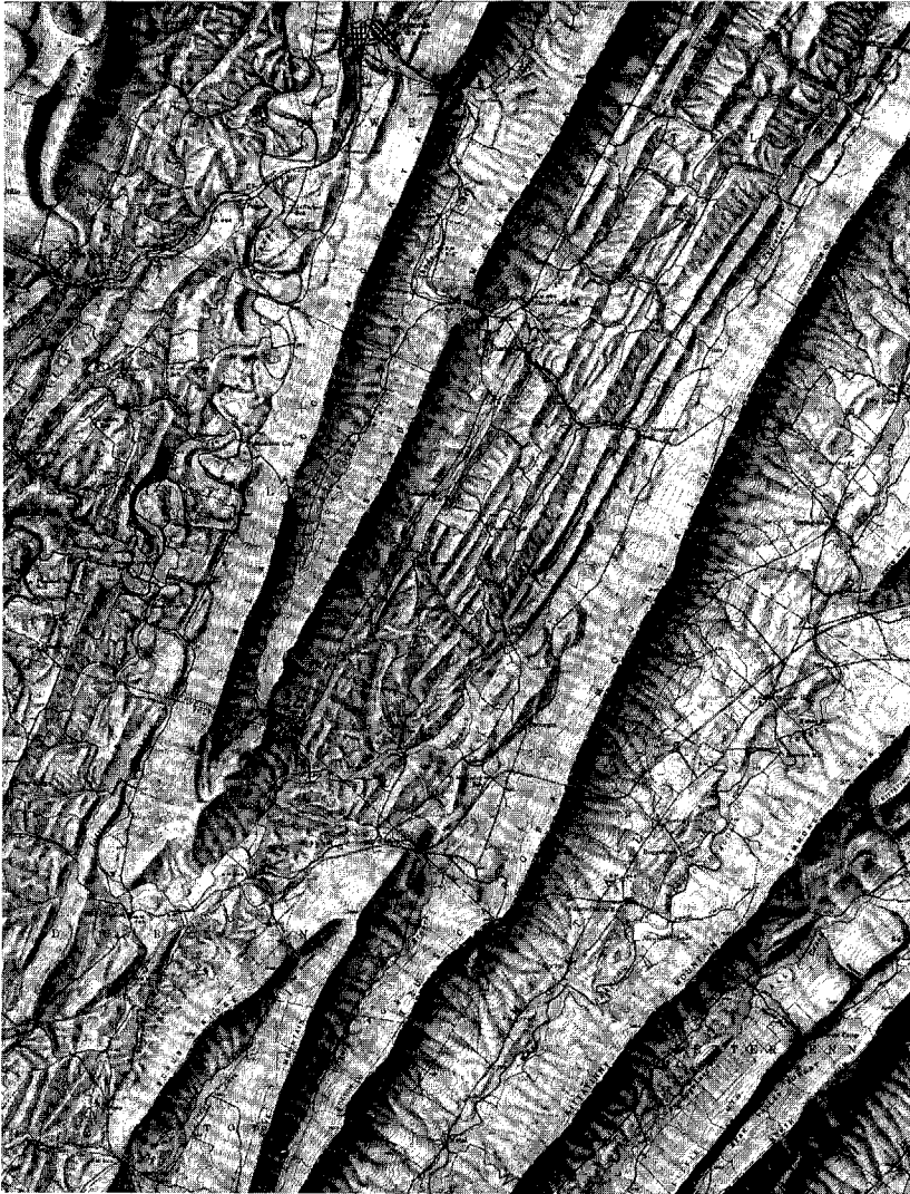
Figure 8.6. Shaded-relief edition of contour map of the area shown in fig. 8.5 (original scale: 1:62,500) by the United States Geological Survey, with marginal data eliminated (reduced).
