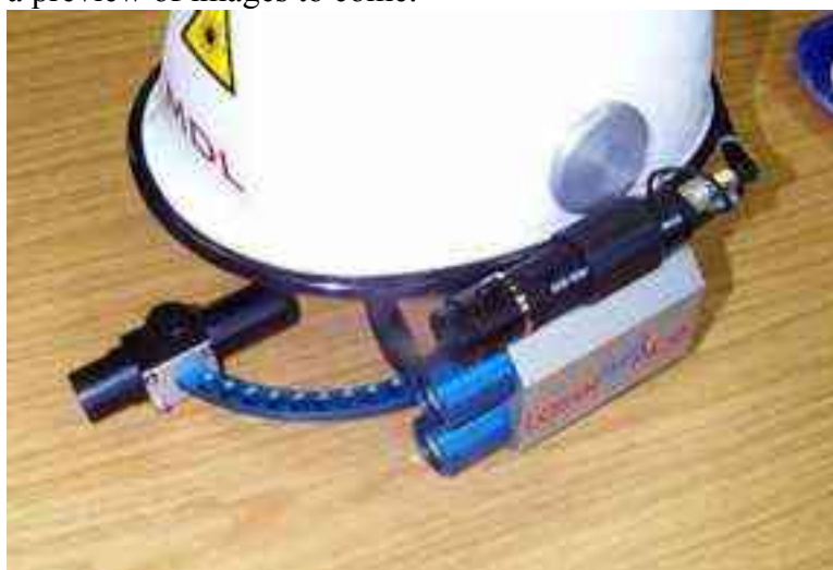
Fig. 15. Hypothetical Future for the system DAIT: a helmet with integrated Telemeter
