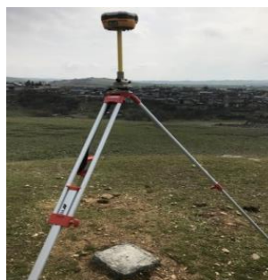
Figure 8: Static measurement of BM1
