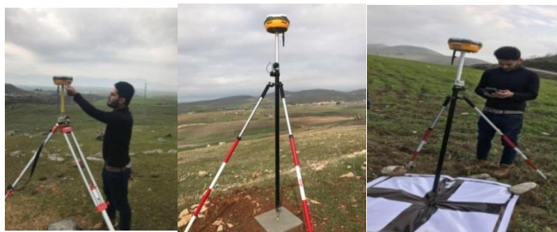
Figure12: RTK measurement of CPs and GCPs
