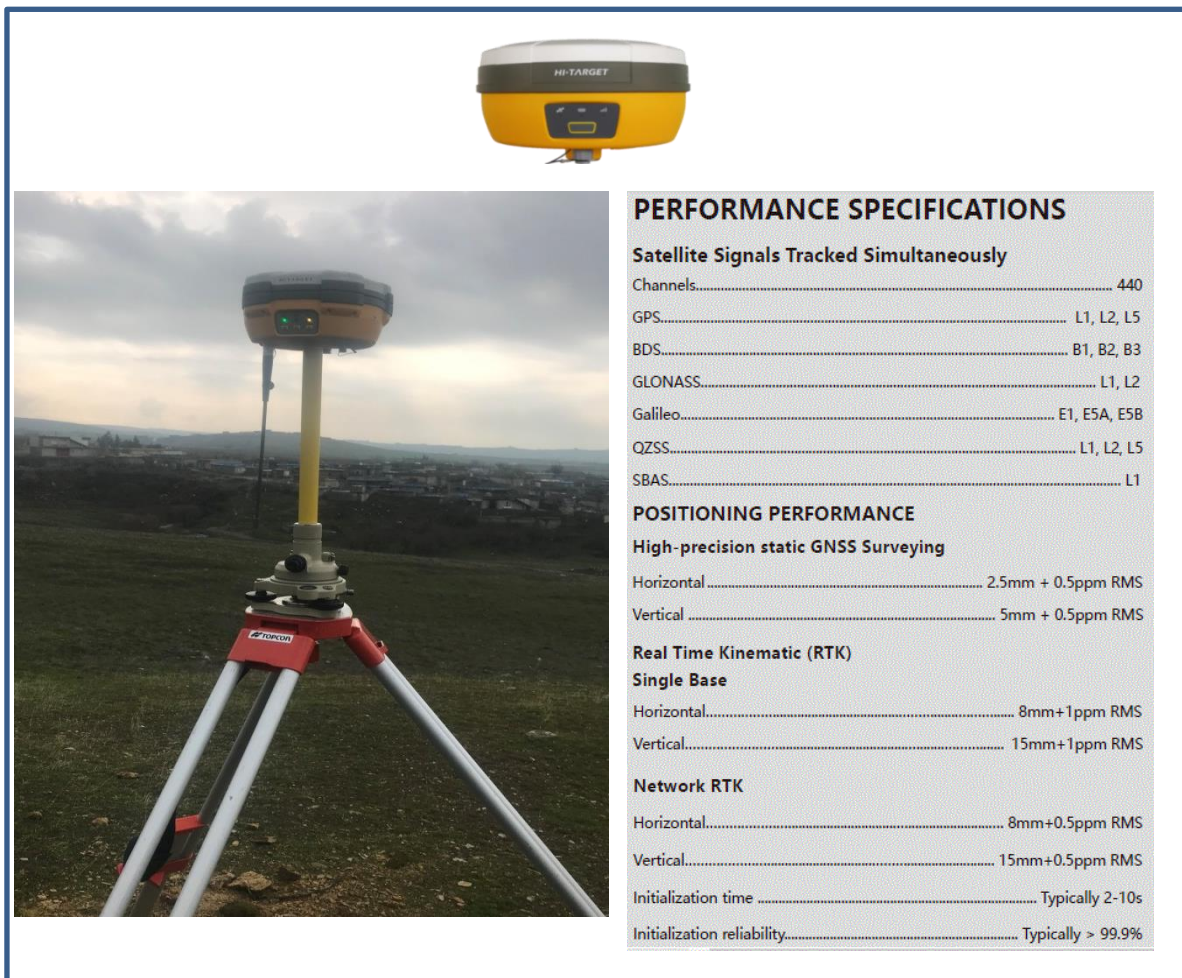
Figure7: HI-TARGET V30 PLUS and specifications (source: equipment manual)
