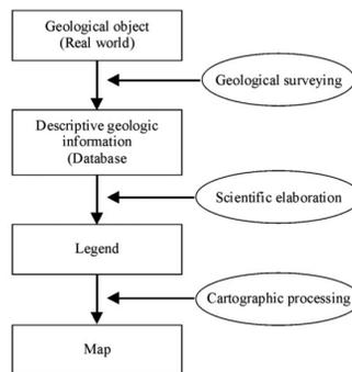
Fig. 1. Model of the geologic map elaboration process
