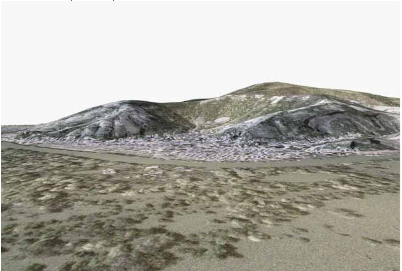
Digital orthophoto of Tokaj, draped to the high resolution DEM
