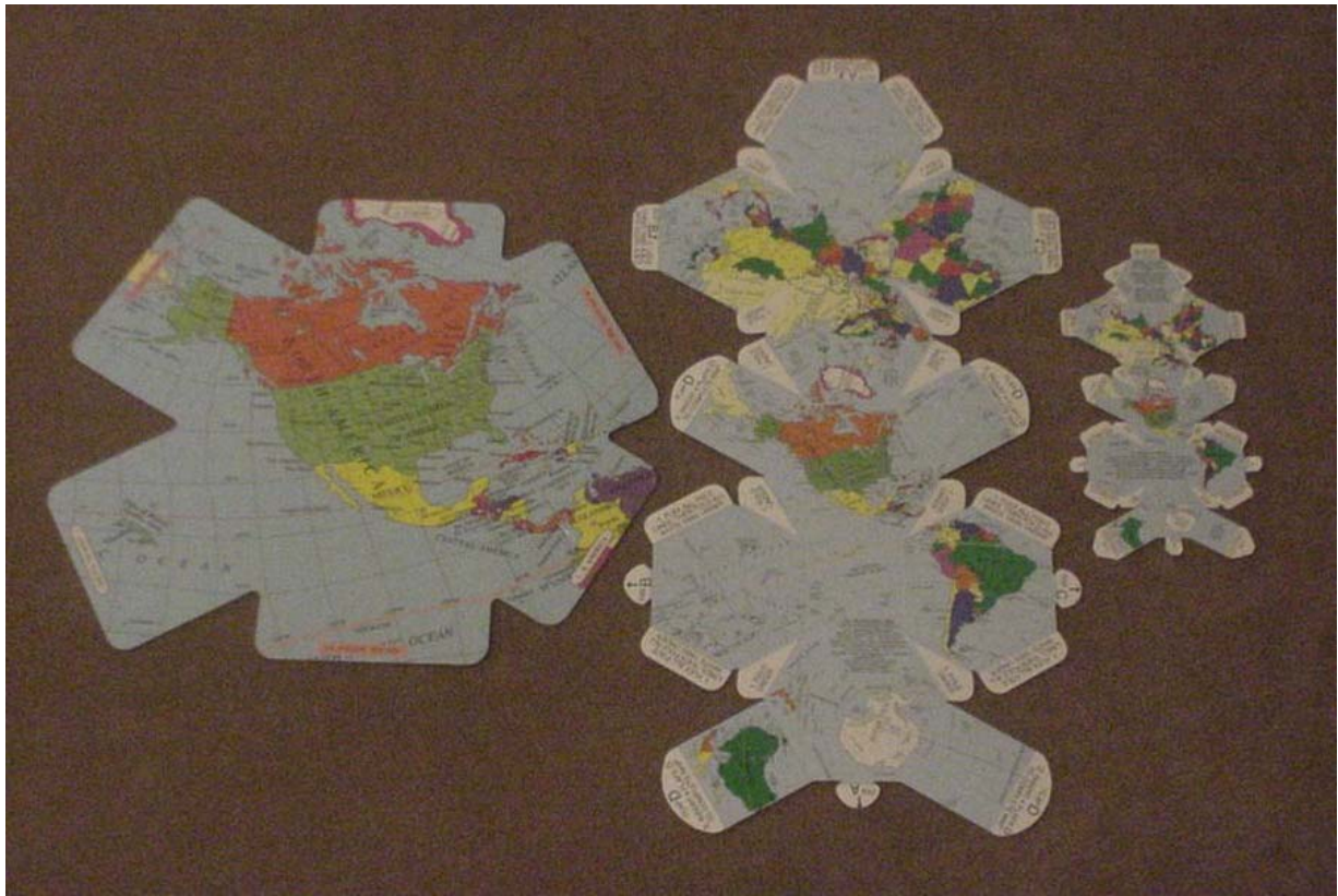
Figure 2. The three sizes of Smith's RealEarth GlobeMap. Note that the shown North America facet of the 30 cm (12 inch) diameter globe has cartographic detail on each of the six tabs (extensions) that are used to join the facets. Three sizes are available: the smallest is like a golf ball and the largest is like a basketball.
