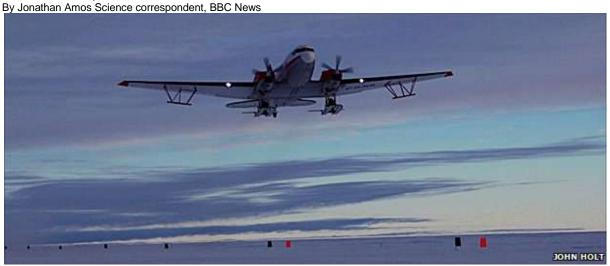
The DC-3 departs from Casey Station. The ice-penetrating radar antennas can be seen under each wing
