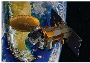
An artist's concept of the Aquarius/SAC-D spacecraft. Instruments on the spacecraft, will take NASA's first space-based measurements of ocean surface salinity. *Photo: NASA*
