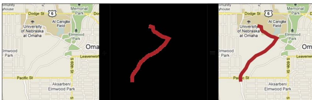
Figure 6. The tile overlay method. A map tile on the left is overlaid with a transparent PNG file with an opaque line. Combining the two tiles produces the display on the right.
