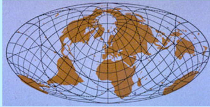
Figure 2: An Oblique Mollweide projection with equal area spherical triangles superimposed. From Fisher and Miller (1944, 75).
