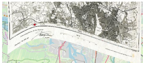
Figure 2. Misplaced GCP because of a recognized place name on the map margin. Transformed Map: TK50 Langenhorn (1909) Background map: OpenStreetMap
